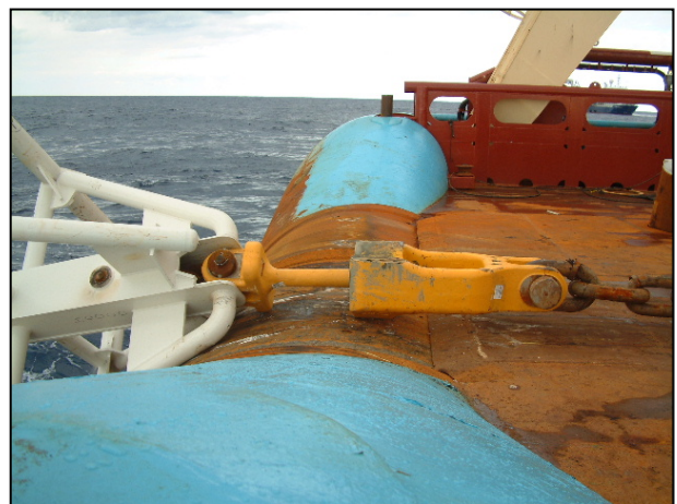
Fig. 4 – deployment of subsea connector and seabed frame
