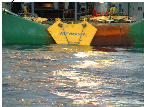
Fig. 7 – anchor deployment of the stern roller
